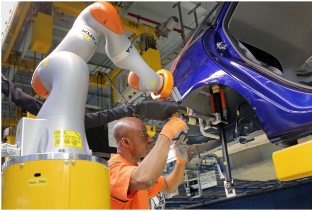
Figure 1 | Cobot application at Ford Motor Company. A cobot application at a Ford Motor Company's assembly plant in Cologne, Germany. In the application, the cobot carries a heavy, air-powered tool, which the worker positions during the installation of shock absorbers in Ford Fiesta model cars. (Copyright: Ford Media Center.)
